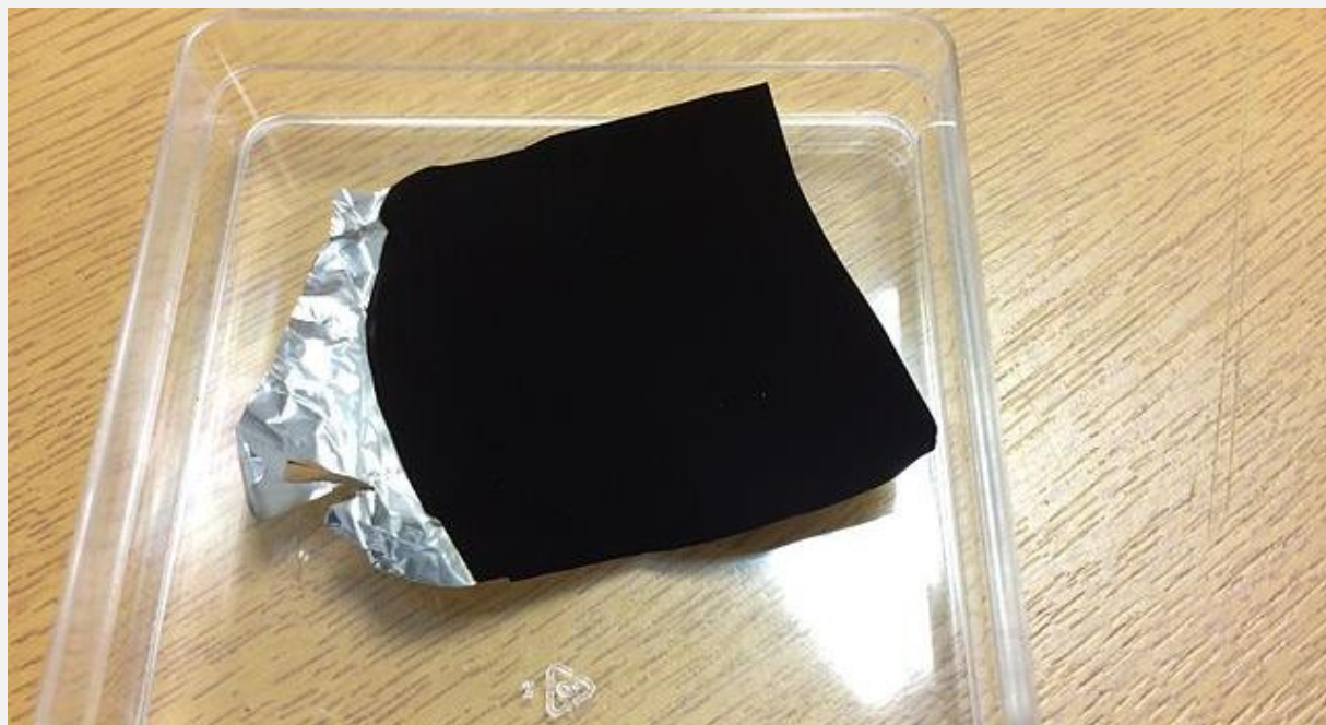
Vantablack grown on metal foil By © Surrey NanoSystems - Surrey NanoSystems, CC BY-SA 3.0, https://commons.wikimedia.org/w/index.php?curid=34139563
